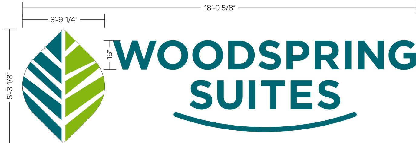
CHANNEL LETTER DETAIL SCALE: 3/8" = 1'-0"
