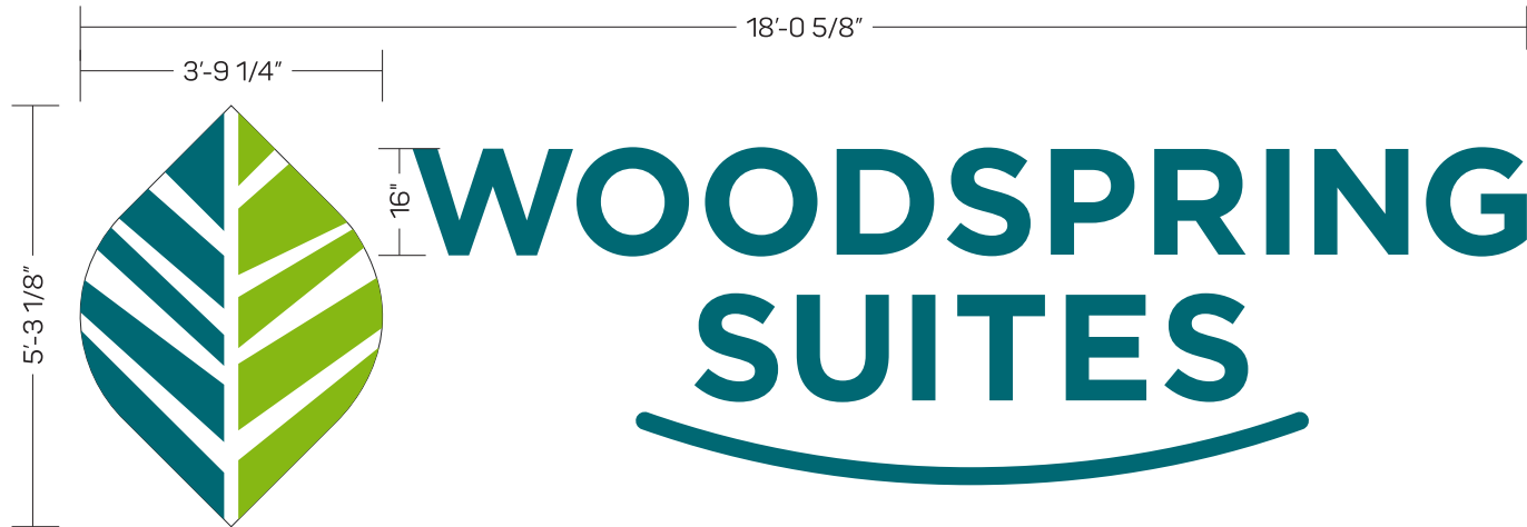
CHANNEL LETTER DETAIL SCALE: 3/8" = 1'-0"
