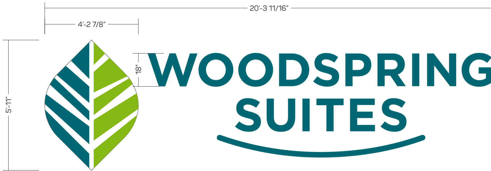
CHANNEL LETTER DETAIL SCALE: 3/8" = 1'-0"
