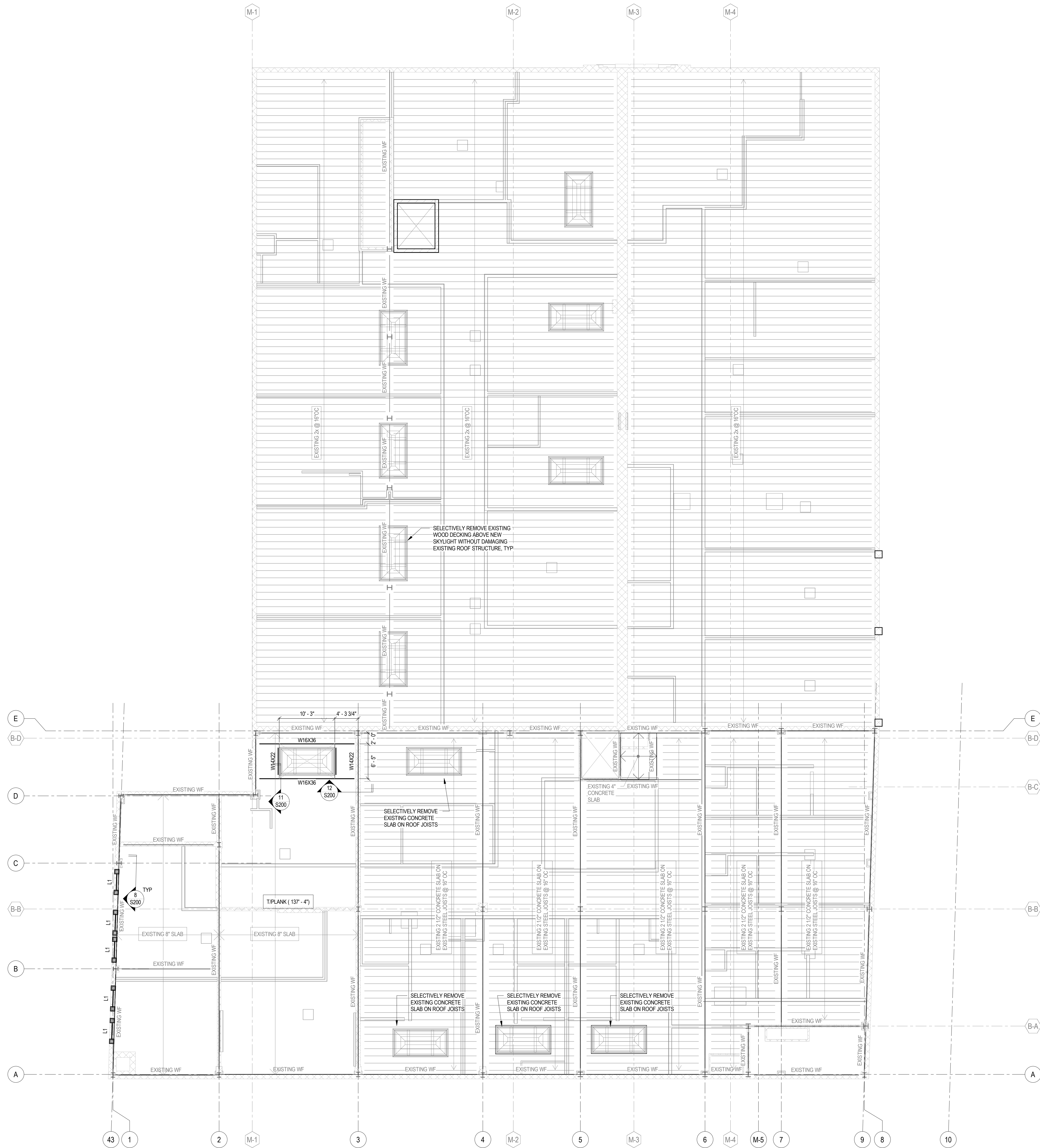
1 S104 ROOF FRAMING LEVEL SCALE: 1/8" = 1'-0"
