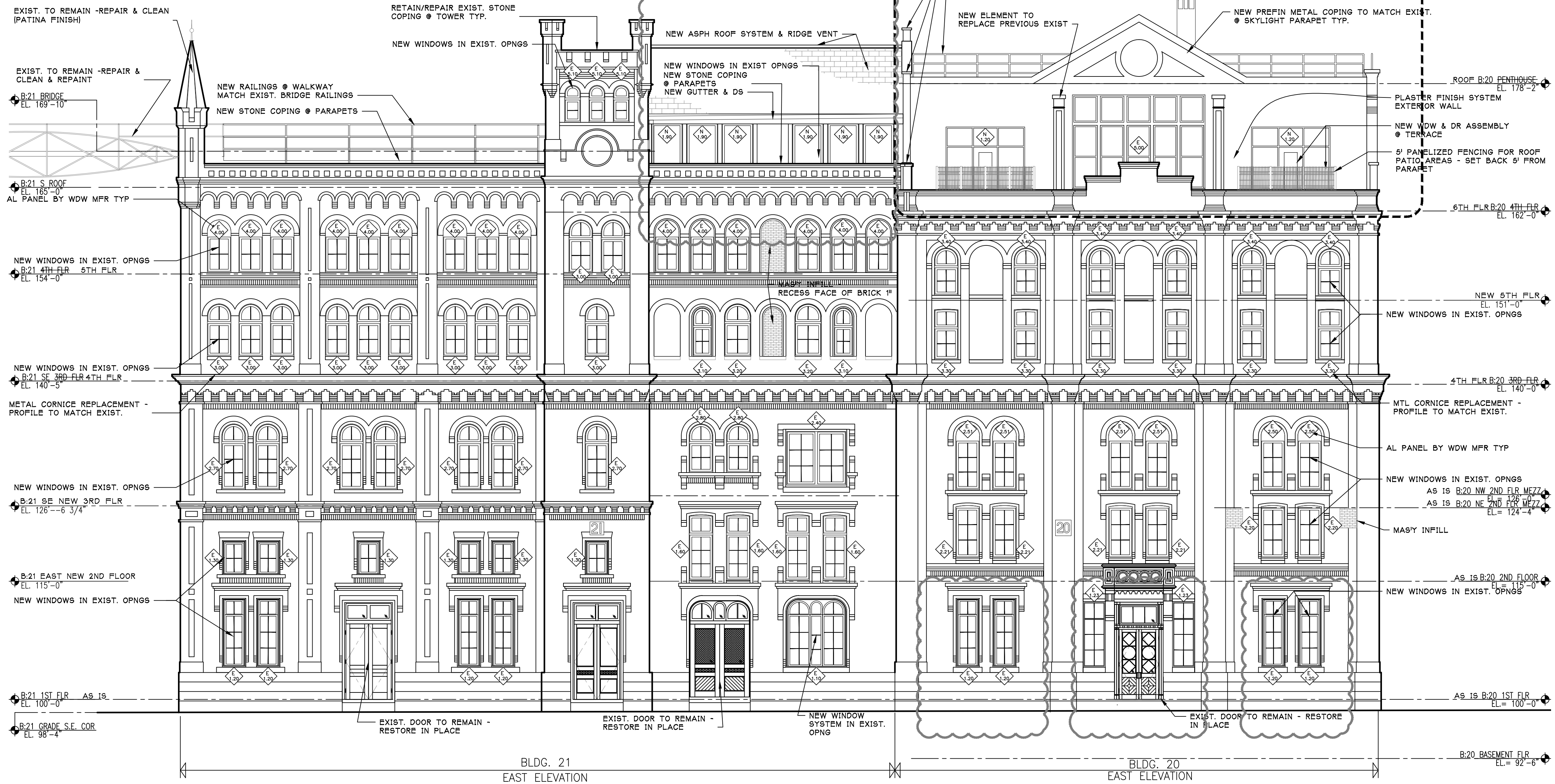
A EAST EXTERIOR BUILDING ELEVATION SCALE: 1/8" = 1' - 0"
