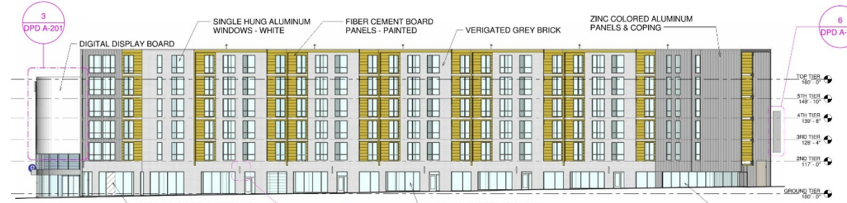
5 WEST ELEVATION WITH HOUSING (DPD)
