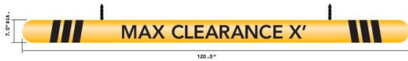
Hanging Clearance Marker 1 / CM1, 7" Dia. Tube, 120" Long, Text & Chain Length TBD QTY: 2 - 1 North Entrance, 1 South Entrance
