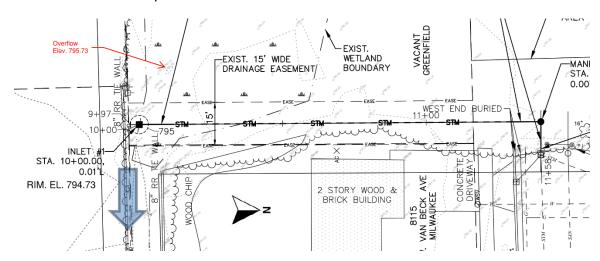
The 5-ac watershed generates approximately 6.5-cfs during the 10-yr event (without accounting for attenuation in the depression). The proposed 15" storm sewer at 0.5% can accommodate approximately 6-cfs which should sufficiently convey the 10-yr event if the depressional capacity was explicitly modeled. Runoff in excess of the storm sewer capacity will continue east as under current conditions.
