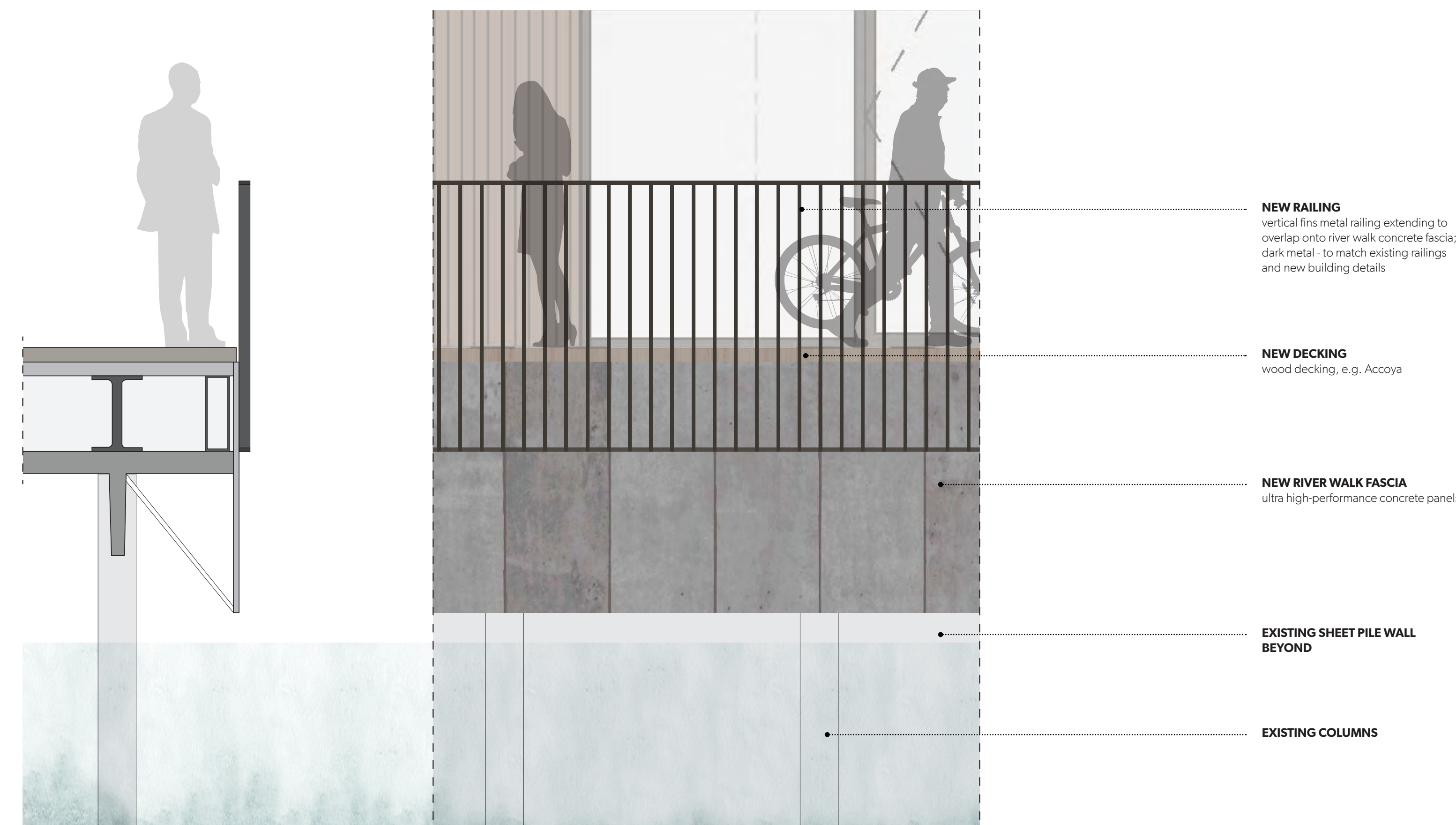
NEW RAILING DETAIL
