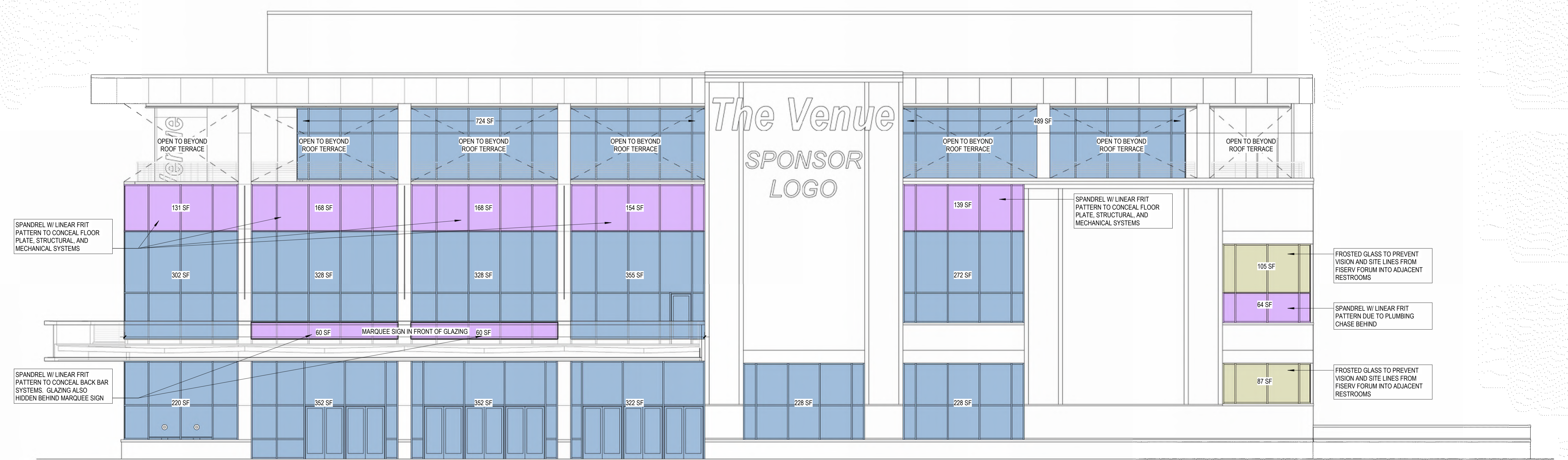
A2 NORTH ELEVATION - GLAZING TYPE ANALYSIS 1/8" = 1'-0"
