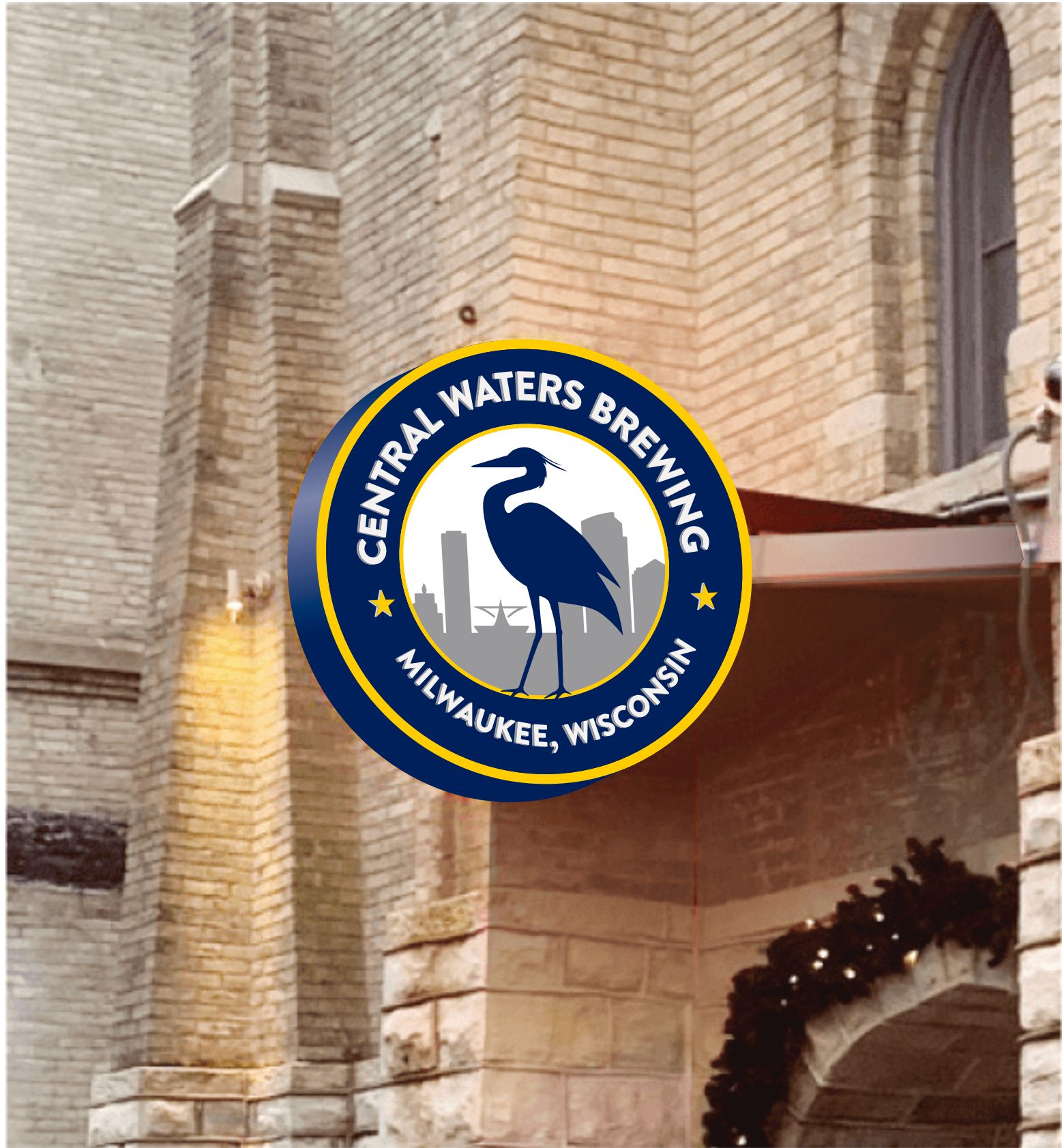
BLADE SIGN-1, BS-1 48" 2 sided Projecting Blade Sign to Replace Existing, .125" Aluminum Outer Ring w/ Push Through Letters & Stars, Translucent White Acrylic Inner Area with Translucent /Opaque Vinyl
