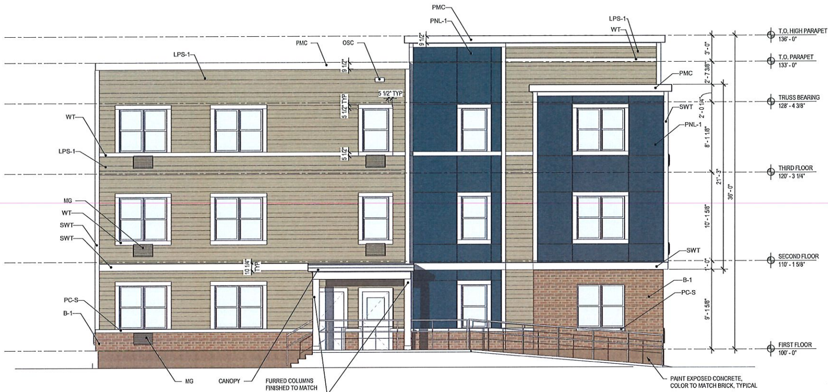
2 EXTERIOR ELEVATION - WEST 3/16" = 1'-0"
