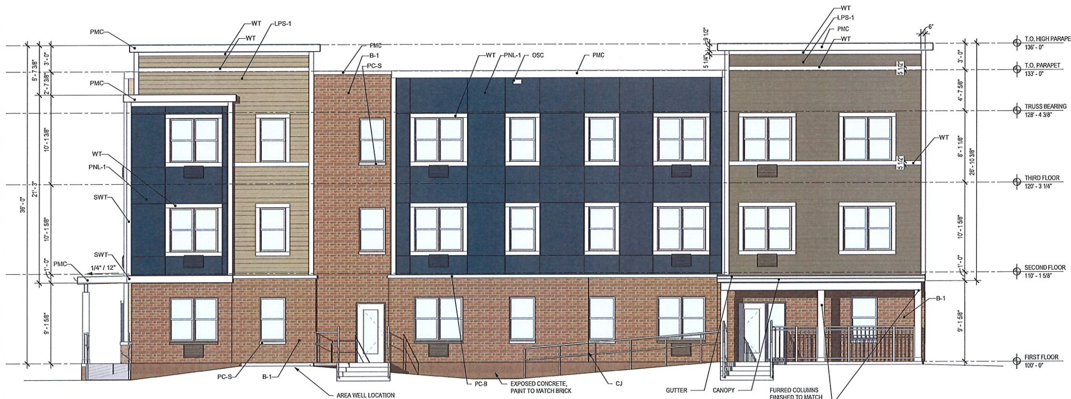
1 EXTERIOR ELEVATION - SOUTH 3/16" = 1'-0"
