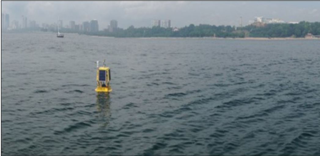
Photo: A buoy at Bradford Beach that is collects continuous water quality parameters to ensure that water quality is safe.
