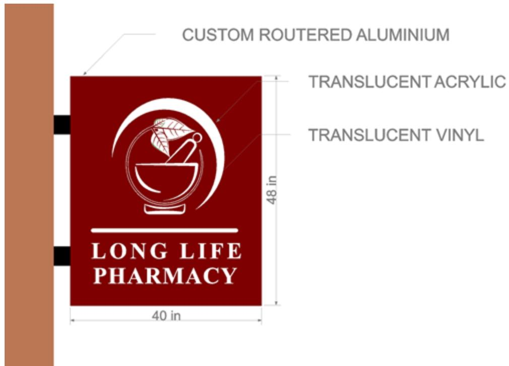
Outermost layer of sign (red) must be opaque.
