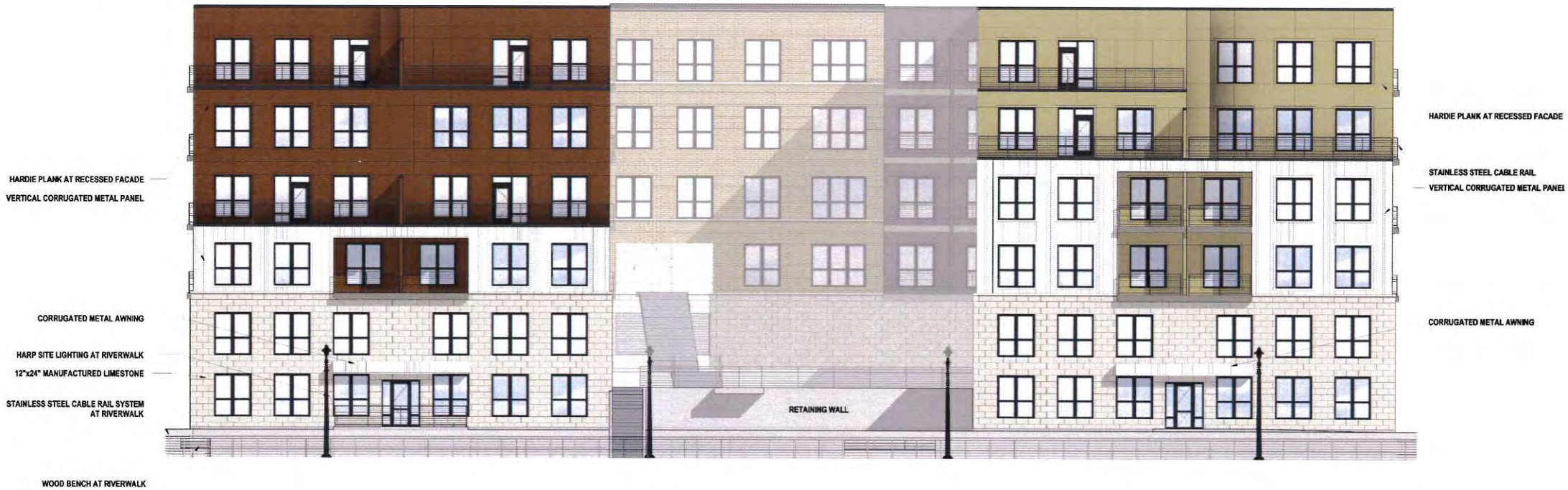
F2 BUILDING 2 - WEST ELEVATION SCALE: 1/8" = 1'-0"
