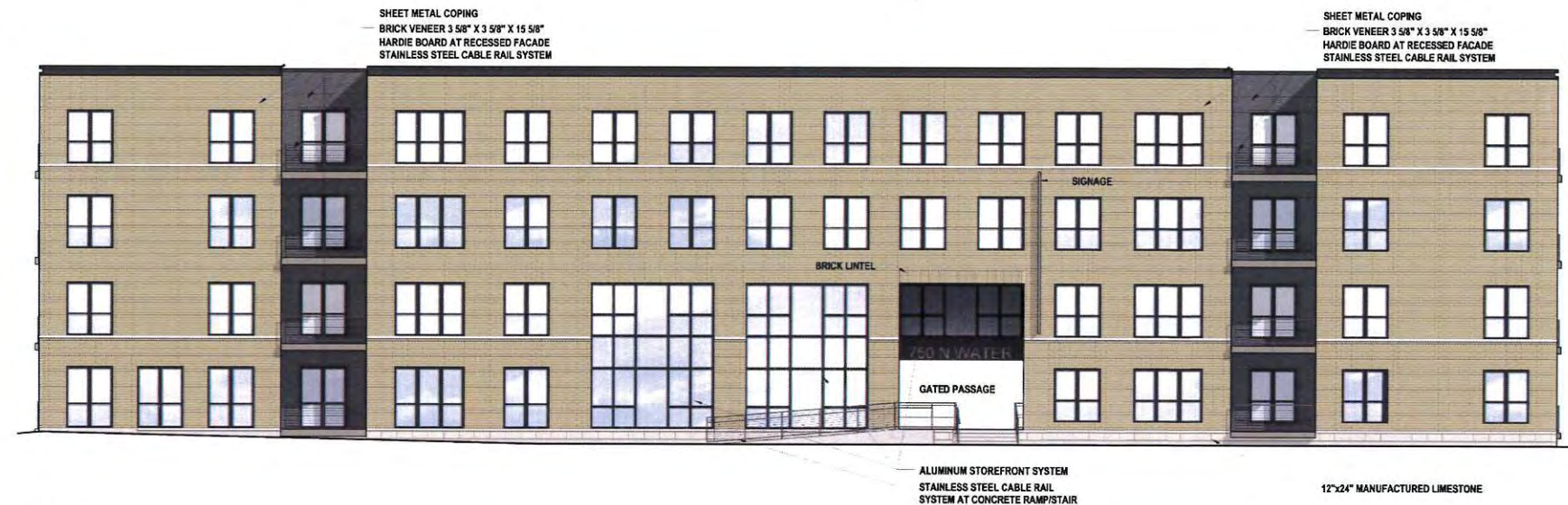
D2 BUILDING 1 - EAST ELEVATION SCALE: 1/8\"/>
