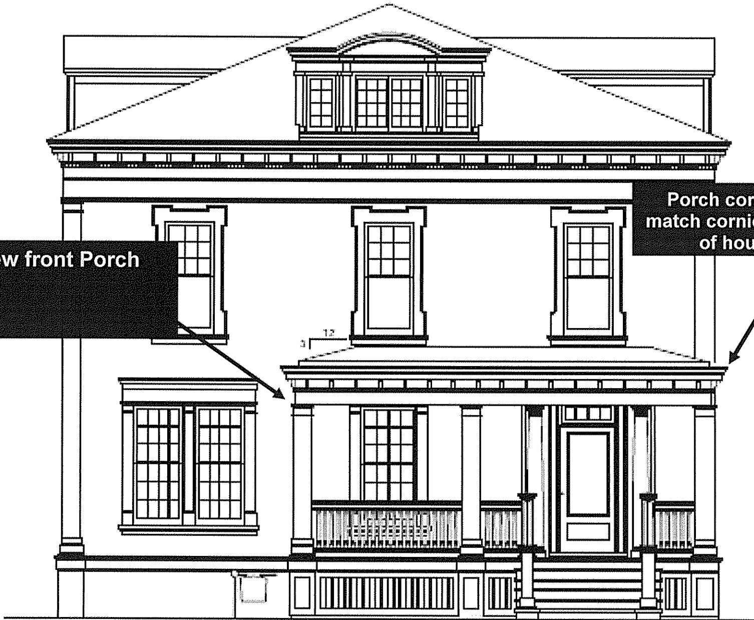
T A1 PROPOSED FRONT ELEVATION w/covered porch Scale: 1/4" = 1'-0"
