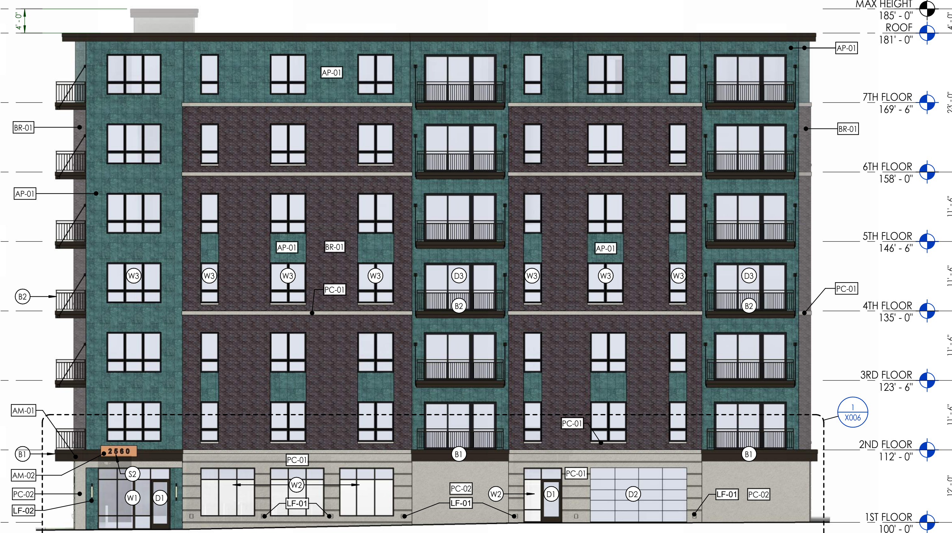
1 | SOUTH BUILDING ELEVATION - EXHIBIT 1" = 10'-0"
