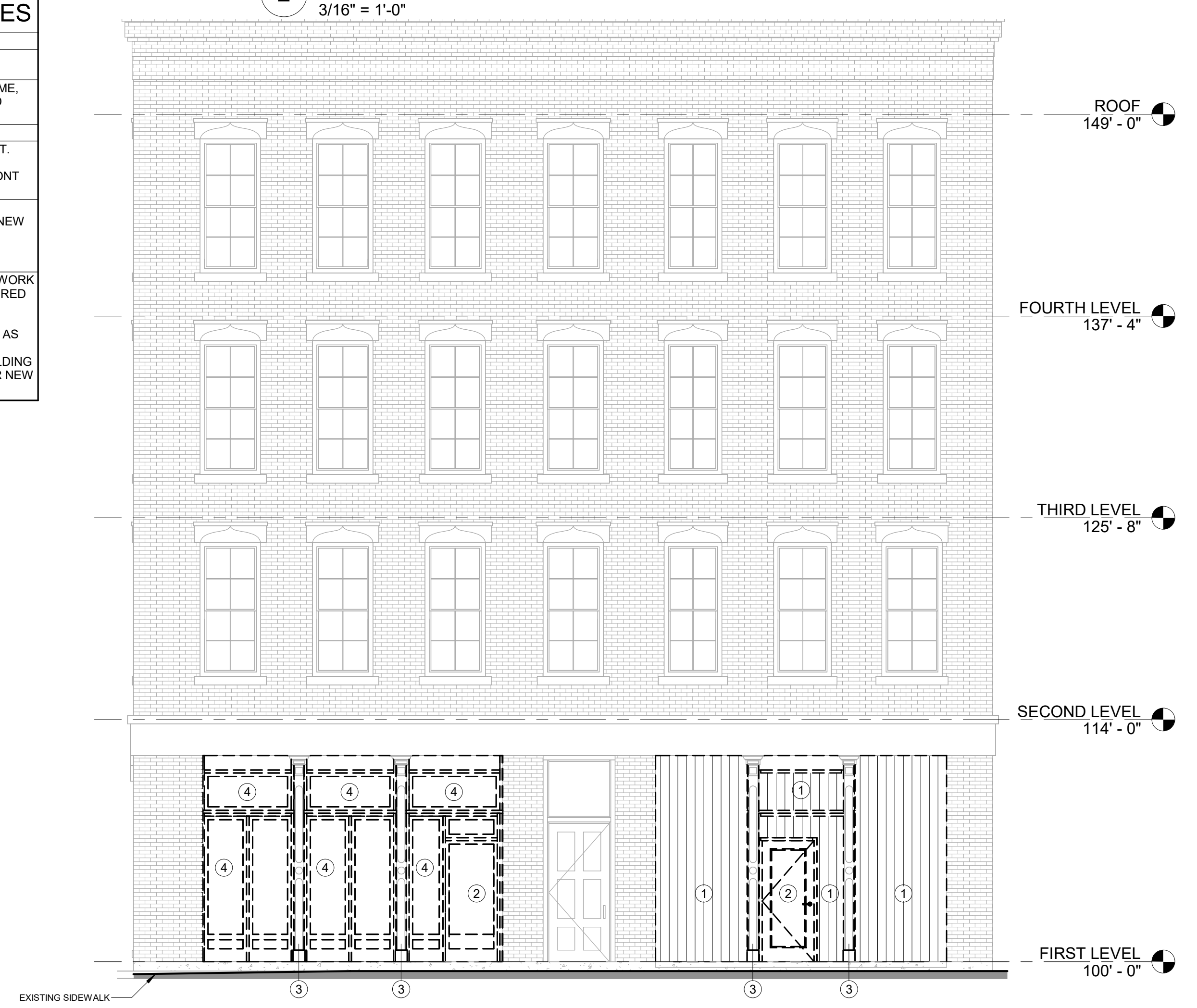
1 DEMOLITION EXTERIOR ELEVATION - EAST 3/16" = 1'-0"
