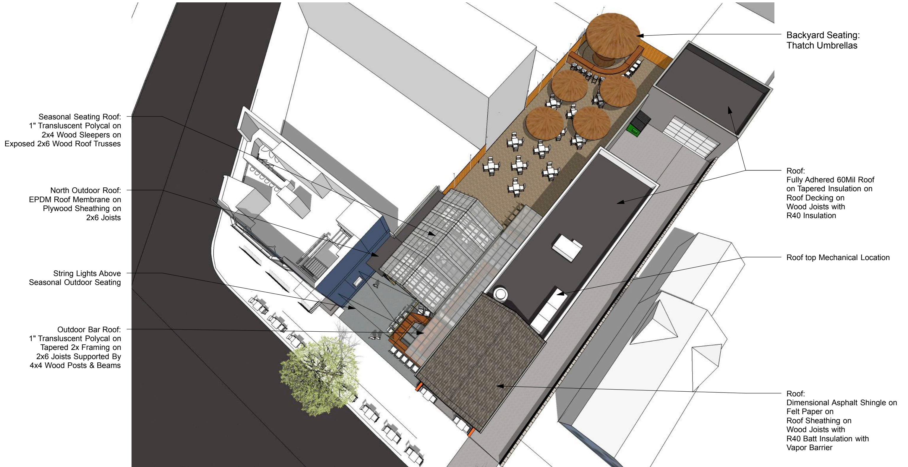
1 A2.2 ROOF LEVEL - AERIAL PERSPECTIVE Scale: NTS
