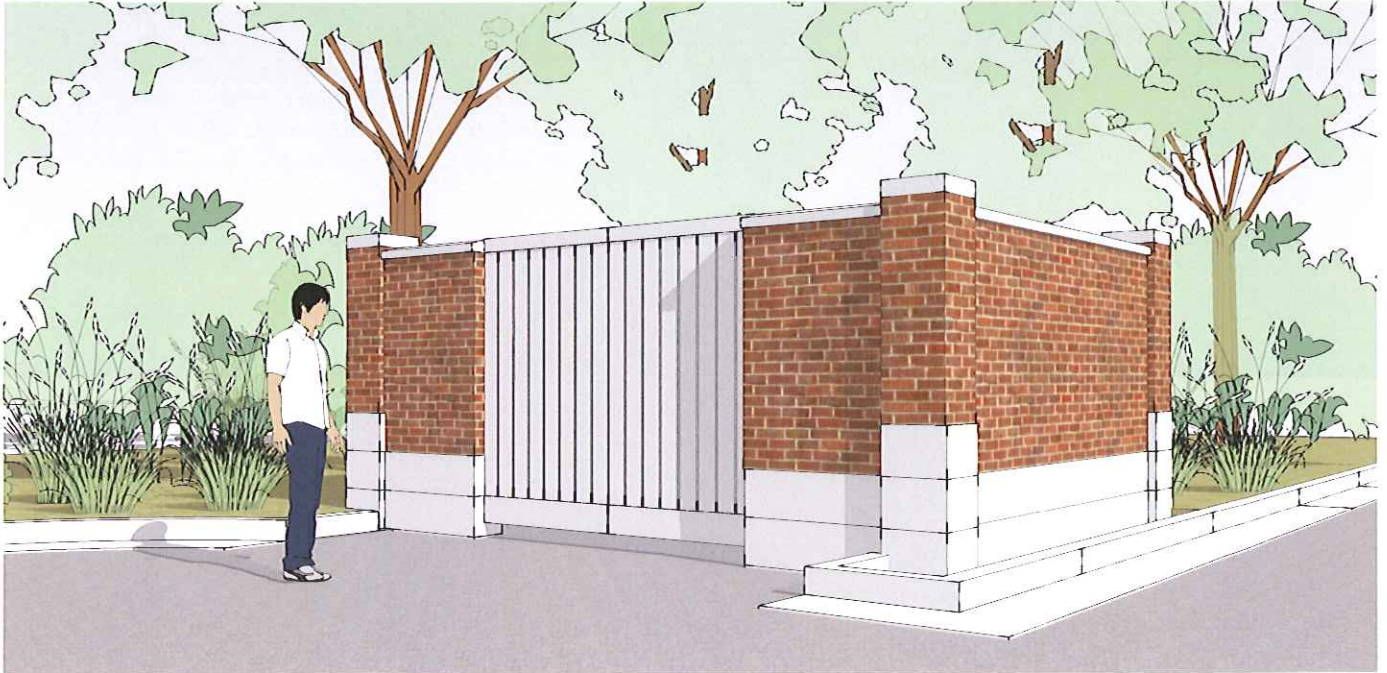
MASONRY SCREEN WALL TRASH ENCLOSURE
