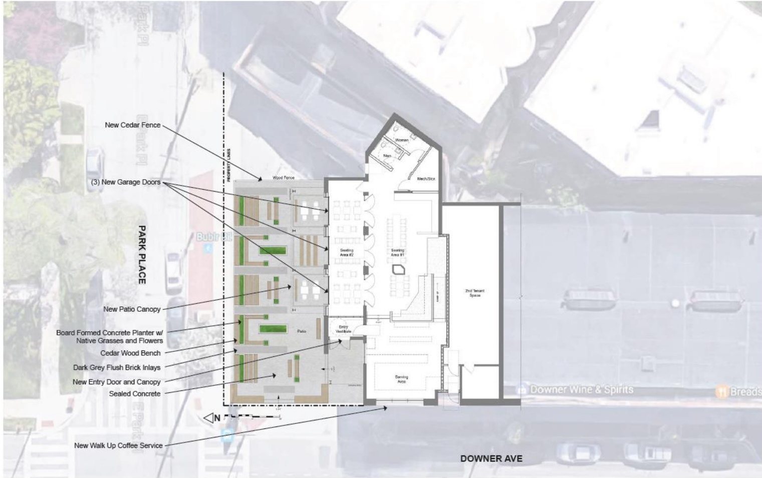
Site Plan / Floor Plan 1/16" = 1'-0"
