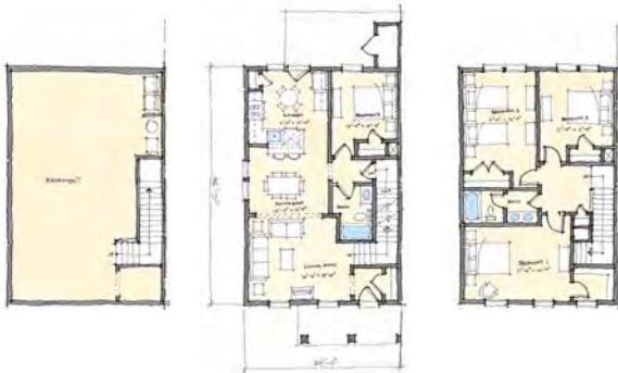
Typical Basement Floor Plan Typical First Floor Plan Typical Second Floor Plan
