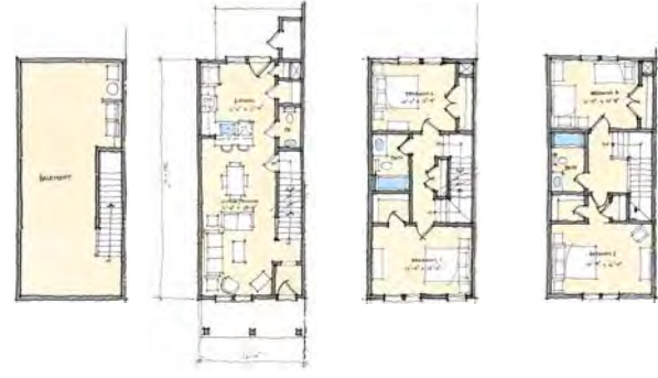
Typical Basement Floor Plan Typical First Floor Plan Typical Second Floor Plan Typical Third Floor Plan
