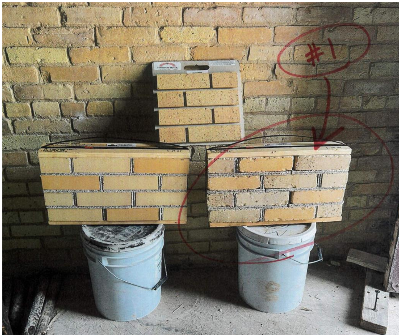
Replacement brick circled. Brick to match as closely as possible the historic cream brick.
