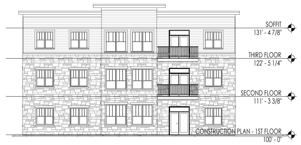
3 SIDE ELEVATION SCALE: 1/16" = 1'-0" (OTHER SIDE ELEVATION IDENTICAL)
