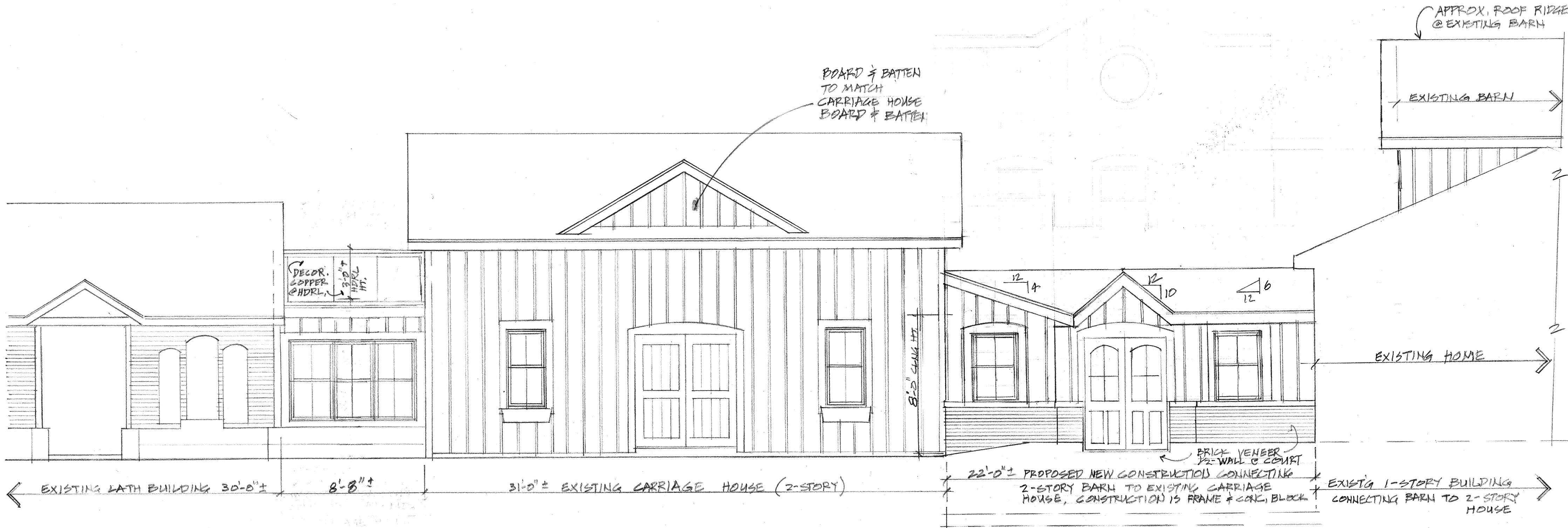
EAST VIEW FRONT ELEVATION 1/4"=1'-0"
