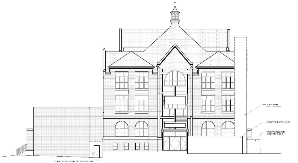
② NORTH DEMOLITION ELEVATION SCALE: 1/8" = 1'-0"
