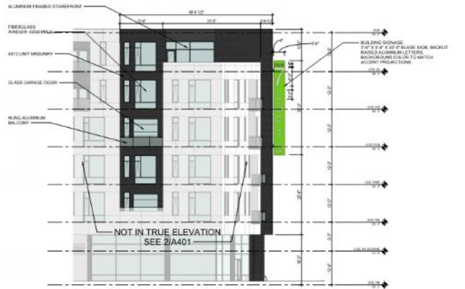
2 WEST ELEVATION - FLAT (SOUTH HALF)
