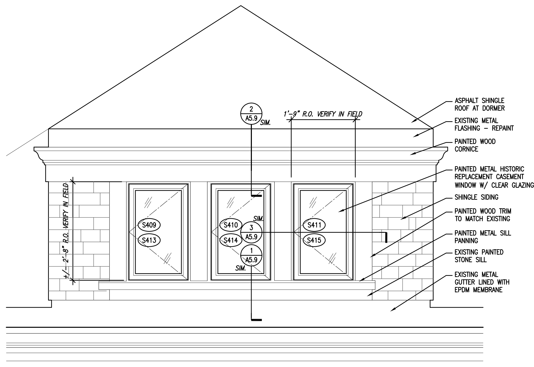
4B TYPICAL ATTIC DORMER WINDOWS AT 1884 BLOCK PROPOSED REPLACEMENT WINDOW ELEVATION SCALE: 3/4" = 1'-0"
