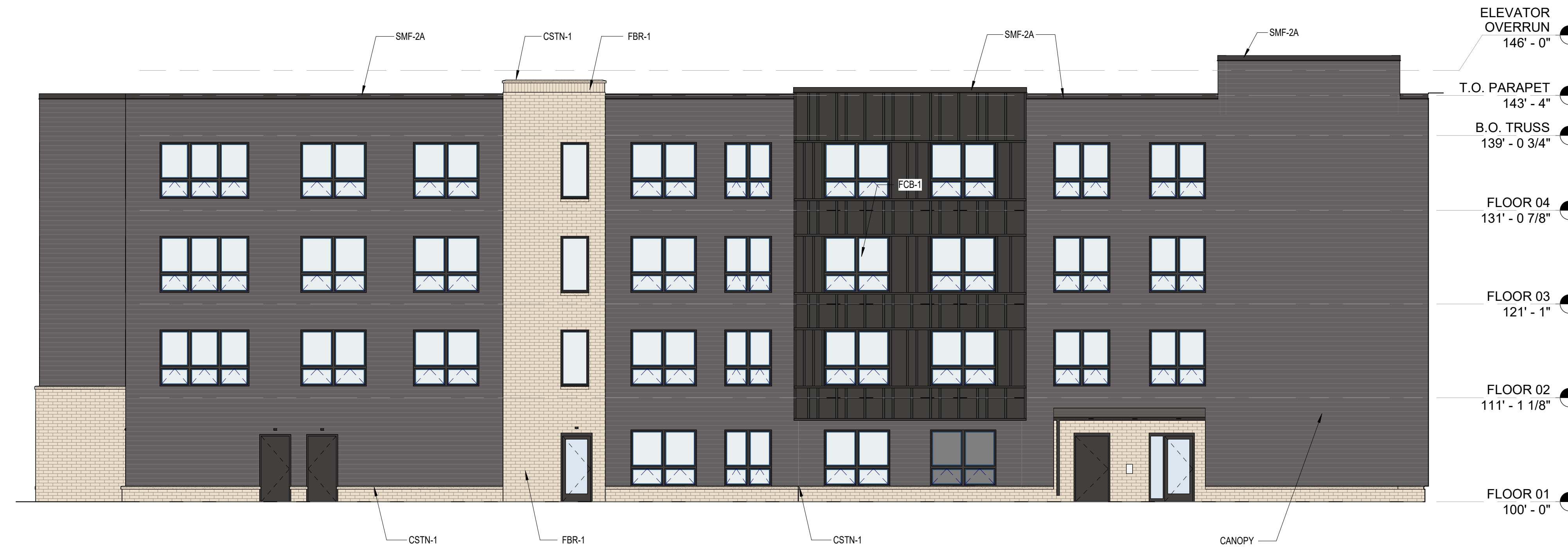
4 COURTYARD - SOUTH ELEVATION (DRT) 1/8" = 1'-0"
