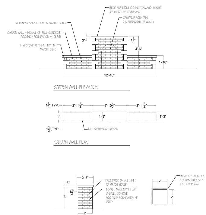
MASONRY PILLAR - PLAN VIEW
