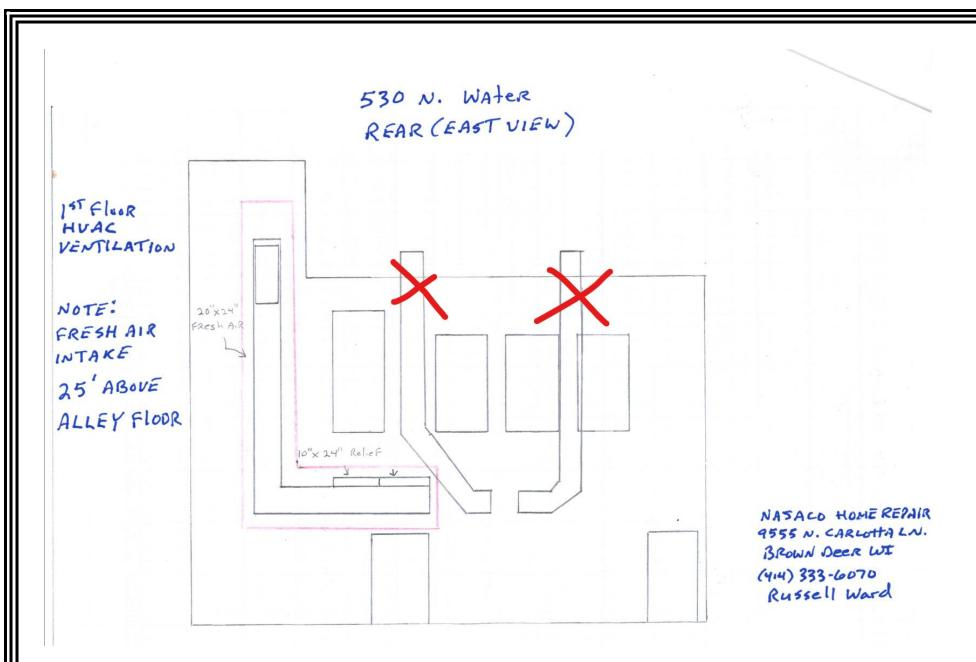
Only the equipment outlined in pink is approved. The two duct stacks at right are kitchen equipment being designed and installed by a different contractor. They must be reviewed indpendently with another COA.
